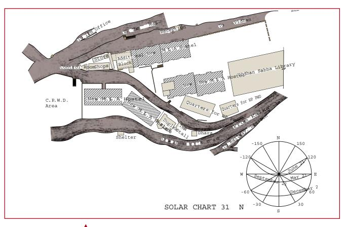
The building blocks in the MIA hostel, Shin a, bcated in the cold and cloudy zone, are oriented due south  $\pm 15^{\circ}$  for direct so larga in. They are spaced aparts o as to eliminate shadows of one building over the other, even for the longer wintershadows. It was proposed that all bedroom s be south facing to avail of the benefit of south exposure
