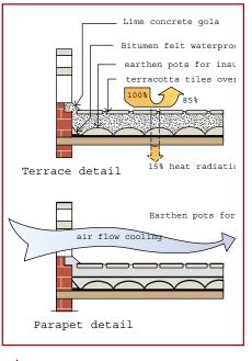
Roofdetails showing use of earthern pots for roof insulation
