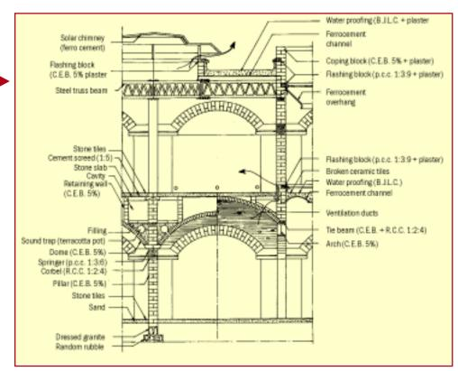
Sectional details showing use of alternative construction techniques. Fenocem ent solar chin ney and ventilation duct in corbelled arch dem onstrates use of passive solar ventilation techniques.
